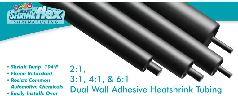
Dual wall adhesive-lined polyolefin heatshrink tubing is ideal for producing strong, weather tight seals on any heatshrink installation. During the application of heat from a heat gun or other heat source, the inner adhesive wall melts and flows, creating an adhesion layer to ensure a snug fit to your harness or connector. Adhesive lined heatshrink comes in 2:1, 3:1, 4:1, and 6:1 shrink ratio, and it is available in 4' sticks.
